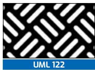
UML 122 Hole: 25mm x 5mm | Pitch: 10mm Open Area: 40%
